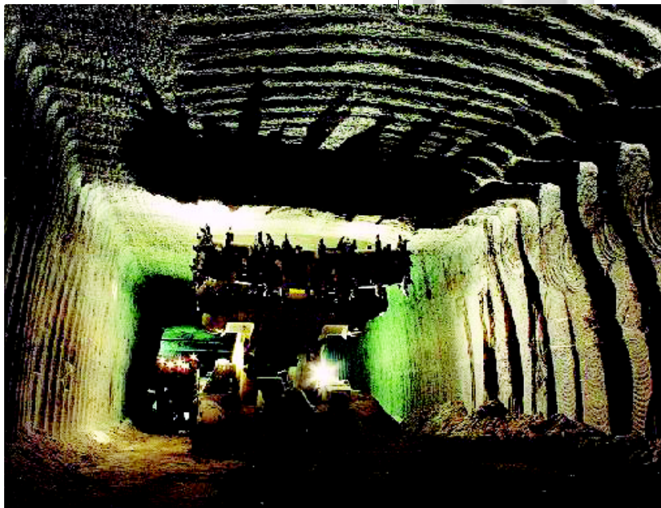
Miners use a Marietta drum miner to cut passages and rooms in the ancient, stable salt deposits. The equipment can mine up to 875 tons per shift.
