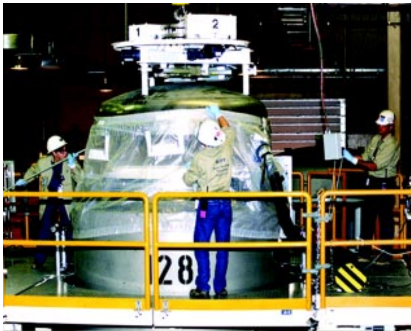
Waste handlers perform a swipe test to check for radioactive contaminants before unloading 55-gallon drums from a TRUPACT-II container.
