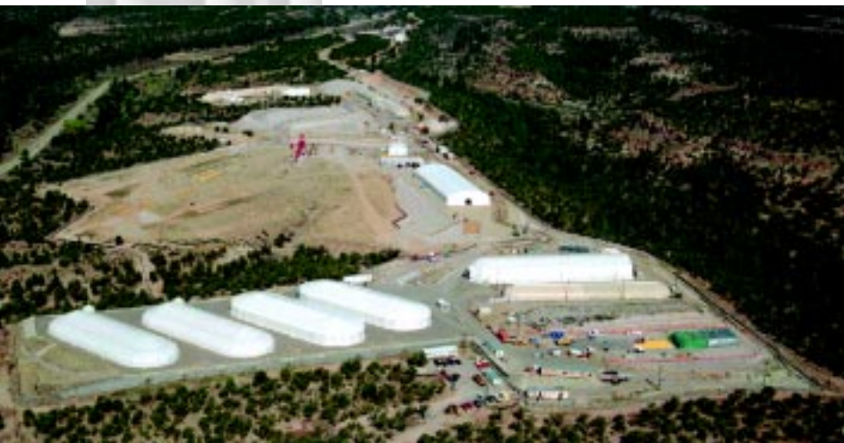
This aerial view of the transuranic waste inspectable storage project (TWISP) shows the six storage domes at TA-54. Since the mid-1990s, thousands of drums of solid mixed and transuranic waste have been retrieved from dense-pack arrays and transferred into the domes, where they are inspected at least weekly, and daily on any day when a staff member enters a given dome.
